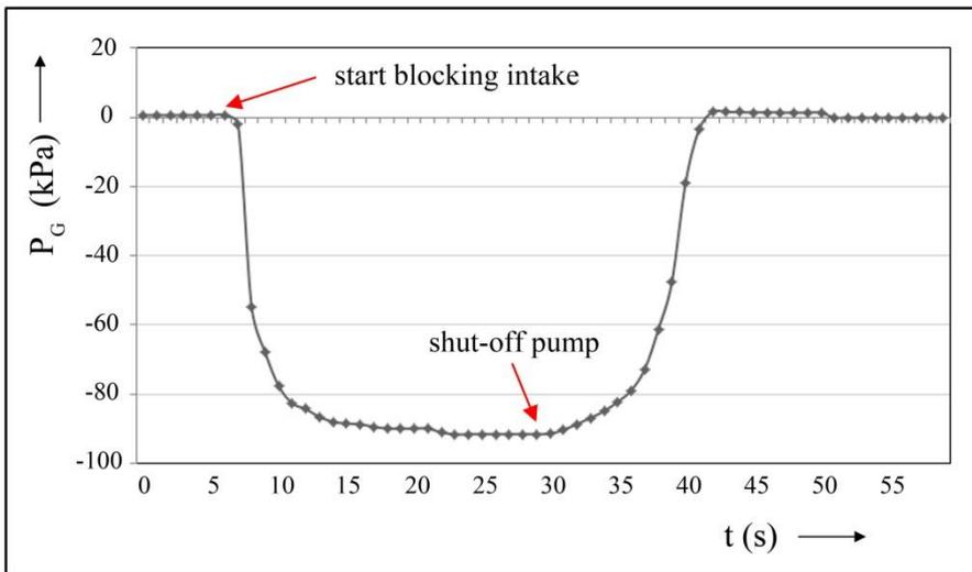
**Figure 6:** Pressure  $P_G$  in time after blocking a single drainage intake at an initial volume flow rate  $Q$  of  $35.6 \text{ m}^3/\text{h}$ .
