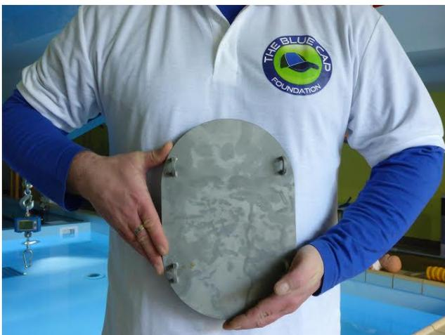
**Figure 7:** Test device of obstruction test as described in European Standard 13451-3. Many commonly used grates in swimming pools cannot be fully blocked by the test device.
