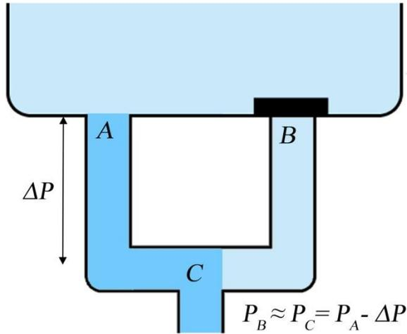
**Figure 2:** The hydrostatic pressure  $P_H$  at a certain depth in the pool and the local gauge pressure  $P_G$  behind a drainage intake. Both  $P_H$  and  $P_G$  are gauge pressures relative to the atmospheric pressure  $P_{ATM}$ .
